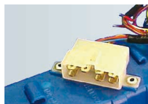
Automotive plastic connector to moulded chassis
